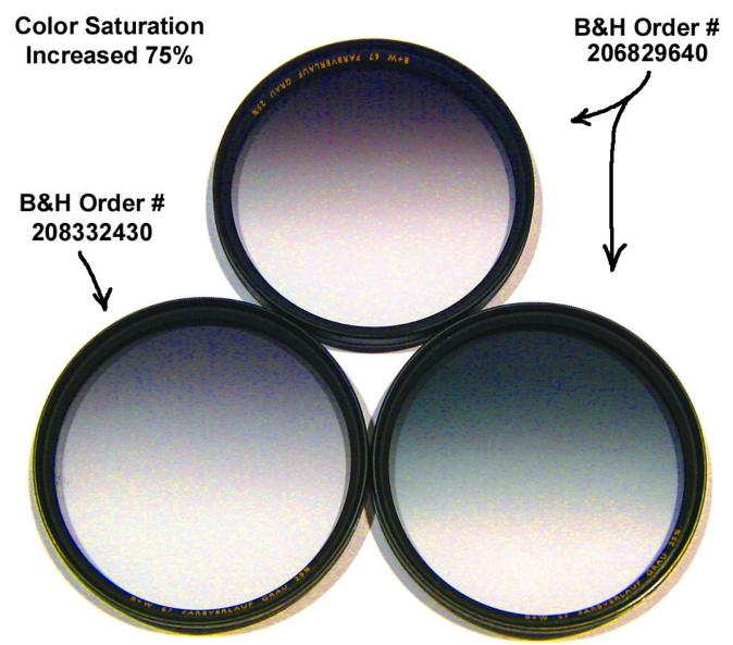
The bottom left filter is the 4th order I've placed having returned the 3rd order. Again I've got three 67mm B+W Graduated ND Filters with no two of them having the same density or color and none of them are truly neutral. This latest filter also has defects at 9 o'clock that can't be brushed or blown away with compressed air.
