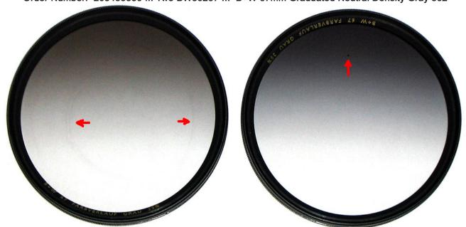
Problem: They have different densities, different color casts, the one on the left has circular smears within the glass, and the other one has a black speck adhered to the surface that can not be brushed or blown off.
