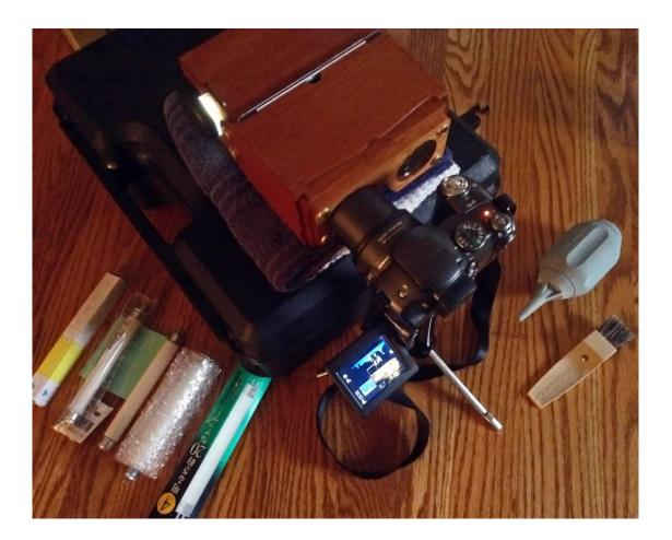
For each of five, six-inch F4T5 fluorescent tubes, rated at different color temperatures, installed in a SaturnSlide<sup>™</sup> Medium Format 3D viewer, a six Megapixel Canon S3 IS was used to photograph only the left-side 50x50mm frame of a mounted medium format stereograph (produced with 120 format Fujichrome Provia 100F, daylight balance, color transparency film).
